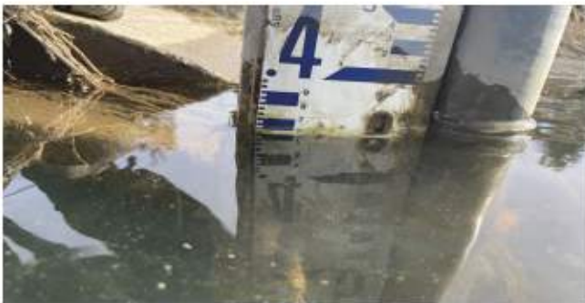
Photo 11: Staff Gauge at Fishtrap Creek Feb 23, 2023
